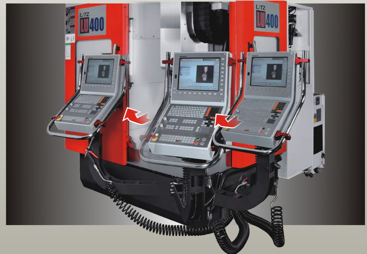
● Adjustable operation panel: it can be operated in front of the machine or at the right-side of the machine. The height of the operation panel can also be adjusted to best-suited the hight of human body.
