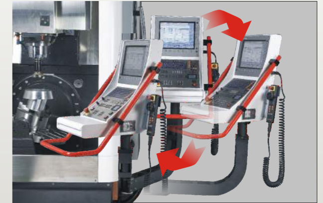
● Movable control cabinet
